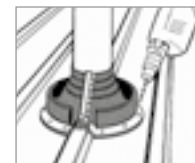
5. Fasten Dektite® with EJOT® self-drilling screws or bulbrite rivets.
