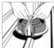
2. Place the Dektite® around the pipe and engage metal teeth in opposing pockets in the sheet starting at the top.
